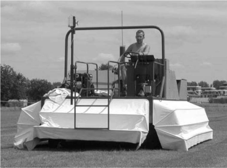
Figure 2. The Inspector Mobile containing two imaging spectrographs and a 3CCD camera in combination with artificial light.
