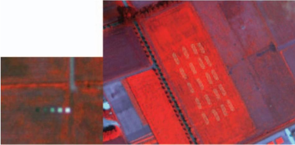
Figure 4. Parts of a false colour composite image made with the UltraCam-D camera over the Wageningen site on 28 July 2004 (image lv102-00234). Left: part of the area with five reference targets is shown, right: the grass/clover test site with the polygons showing the Inspector measurement sites.
